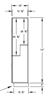
(BASES ARE MADE OF INDUSTRIAL GRADE ' PARTICLEBOARD AND ARE COVERED IN A DURABLE BLACK LAMINATE. PLEASE SET BASE TO ALLOW 5%" BETWEEN THE BACK OF THE LOCKER AND THE WALL FOR AIR VENTILATION.)
