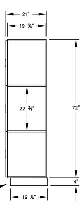
(BASES ARE MADE OF INDUSTRIAL GRADE 1 PARTICLEBOARD AND ARE COVERED IN A DURABLE BLACK LAMINATE. PLEASE SET BASE TO ALLOW %" BETWEEN THE BACK OF THE LOCKER AND THE WALL FOR AIR VENTILATION.)
