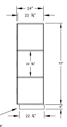
DURABLE BLACK LAMINATE. PLEASE SET BASE TO ALLOW %" BETWEEN THE BACK OF THE LOCKER AND THE WALL FOR AIR **VENTILATION.)**
