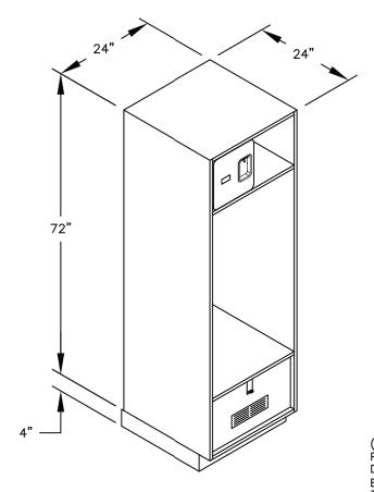
(BASES ARE MADE OF INDUSTRIAL GRADE PARTICLEBOARD AND ARE COVERED IN A DURABLE BLACK LAMINATE. PLEASE SET BASE TO ALLOW %" BETWEEN THE BACK OF THE LOCKER AND THE WALL FOR AIR **VENTILATION.)**
