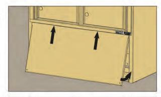
Secure the lower-front panel to the cabinet using a #2 square-tip 1/4" hex-shank insert driver bit and the two (2) screws removed at the start of the installation.
