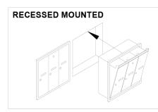
Units fit into a rough opening and are secured with mounting hardware through the back or side panels of the unit. Recessed units include a flanged collar which fits over the rough opening. (Hardware not included.)
