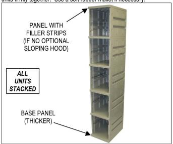
**Step 8.** Insert one (1) of five (5) divider panels in between each of the horizontal panels previously installed. The panels slide in grooves in the side panels and may need the use of a soft rubber mallet to fully engage the two small latch pins into the holes in the front edge of the side panels.
