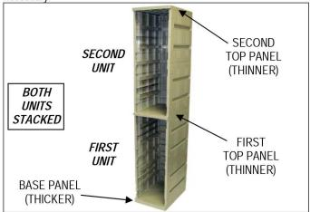
**Step 8.** Install screws and hole covers where side panels join to top panels and base panel. There are 18 screws and hole covers on each side of the two sides of the assembly (36 in total).
